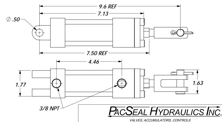
Assembly, Hydraulic Cylinder 2-Pos, 2-1/8" Stroke
